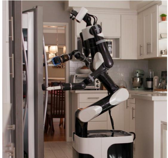
Fig. 1: The general purpose mobile manipulation robot (described in [4]), which consists of a wheeled chassis, torso, left arm, right arm, and head, with a total of 31 DoF. The robot is shown here retrieving an item from a refrigerator, in a home.
